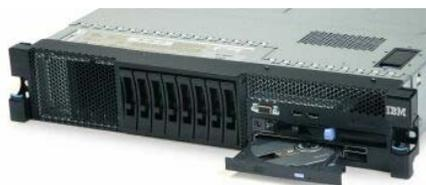
The x3650 M2 contains twelve drive bays in all. Hot-swap drives may be inserted or removed through the front of the server without powering off the system. Simple-swap solid-state drives can be inserted or removed through the front of the server as well; however, the system power must first be turned off.
